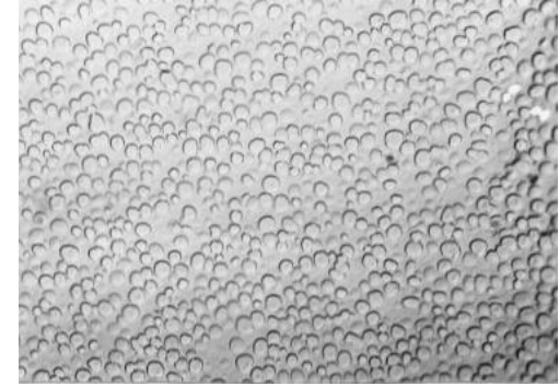
spherical shape of \gamma' -particles
