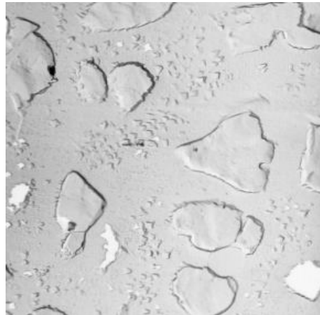
coagulated \gamma' - particles
