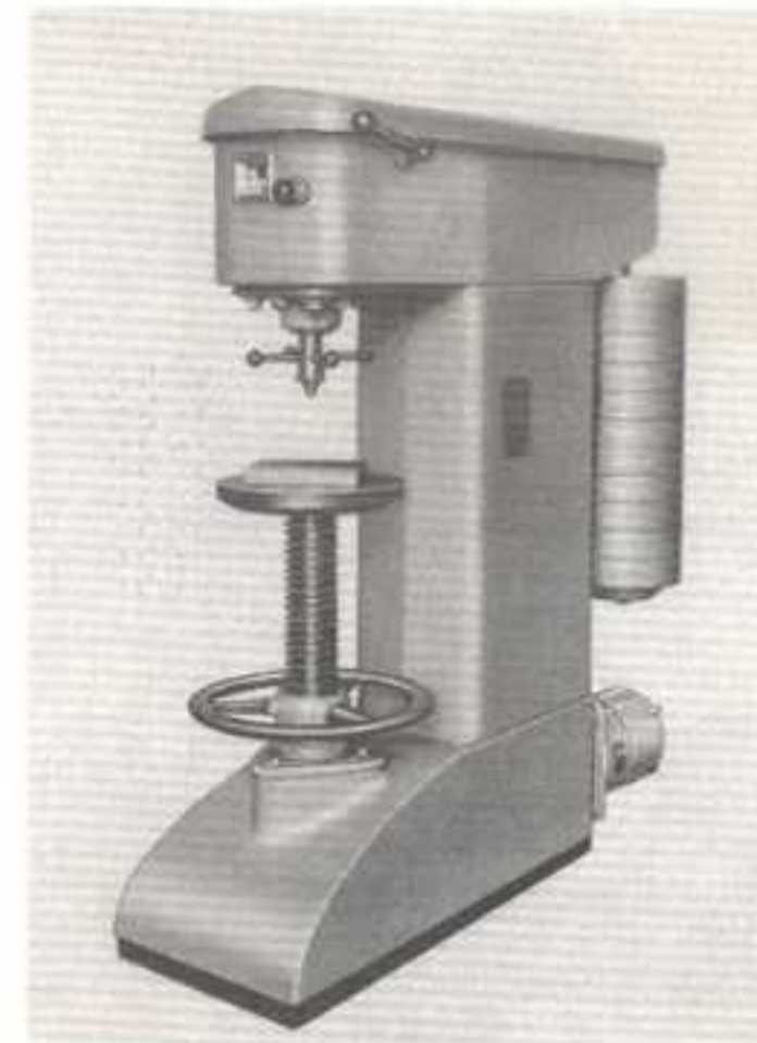
Fig. 46 A Brinell hardness testing machine. (Courtesy Avery-Denison Ltd).
