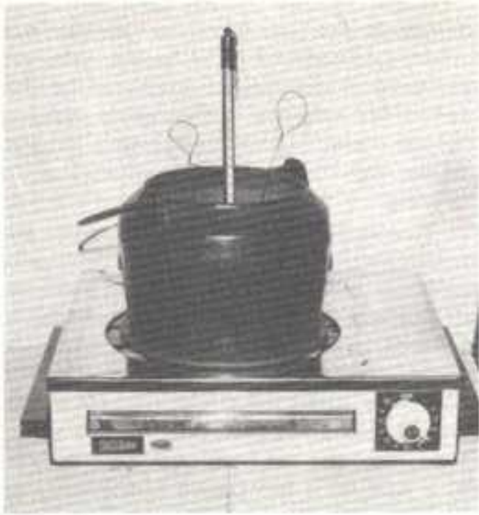
Fig. 20 A simple tempering salt bath. The outer case of a cast-iron glue-pot is set on an electric boiling ring. Note the protective case on the thermometer. Normally a glass-fibre insulating blanket is wrapped round the pot, but was removed for the photograph.
