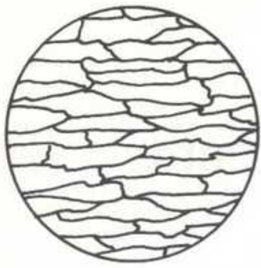
Fig. 40 Elongation of the grains of steel caused by mechanical forming processes.
