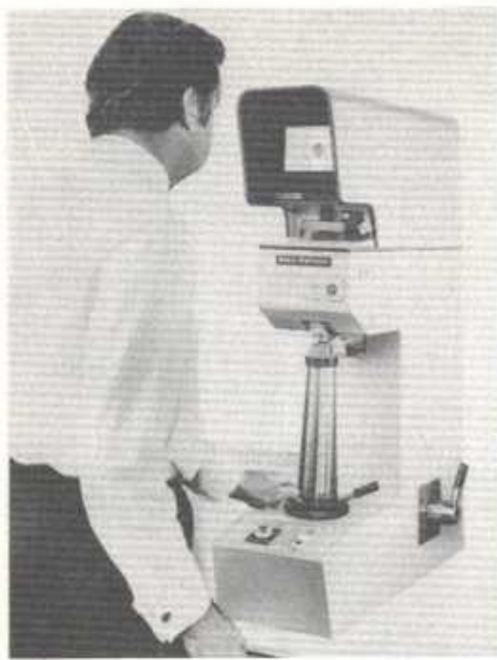
Fig. 48 A Vickers type hardness tester. This machine has a projector microscope which throws an enlarged view of the impression on a screen. (Courtesy Avery-Denison Ltd.)
