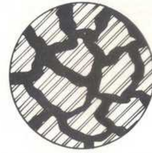
Fig. 14 Grains of Pearlite surrounded by borders of Iron Carbide (Cementite).
