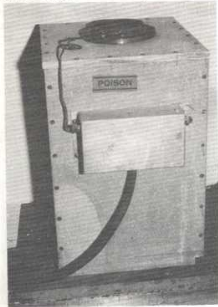
Fig. 34 The author's laboratory type Austenising salt-pot furnace. Construction is described on page 98. Note that the "POISON" label refers to previous use with a cyanide hardening pot.
