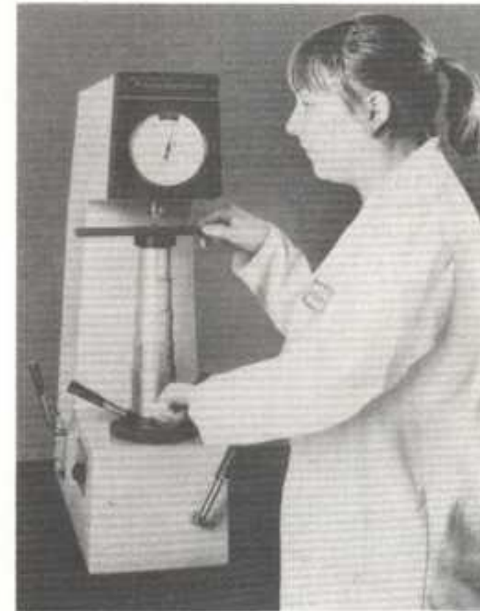
Fig. 47 Hardness testing using a Rockwell type machine. The depth of the impression is shown on the large dial indicator. (Courtesy Avery-Denison Ltd).
