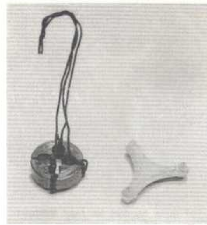
Fig. 28 Method of holding a screwing die for quenching, with a trivet on which it is supported during heating on the right.
