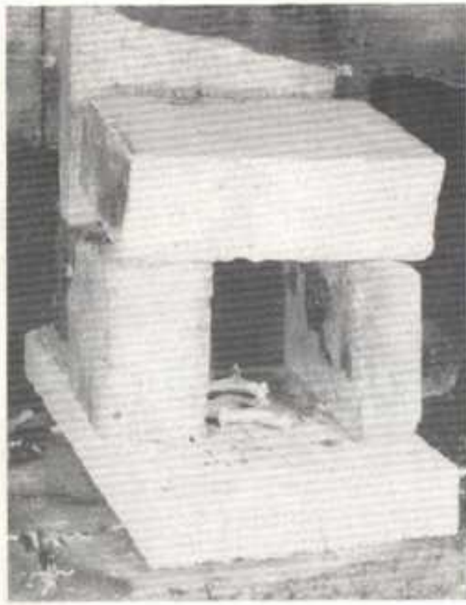
Fig. 27 A crude but very effective heat conserving device. The hot gases escape between the back and top bricks. Note the little ceramic trivets for supporting the work.
