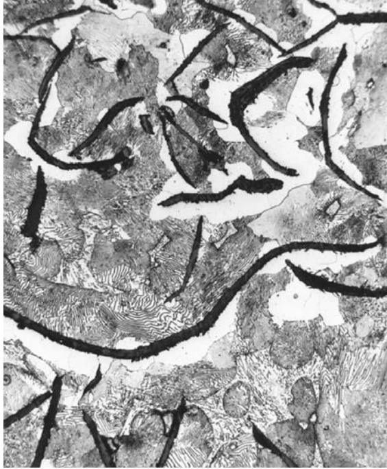
Fig. 16.9 Gray iron with a ferrite-pearlite matrix. Original magnification: 250x
