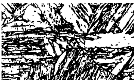
Fig. 4.3. A steel 18XH4BA microstructure after normalization: martensite (dark plates) and residual austenite
