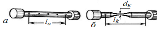
Fig. 1.4. The sample before test (a) and after the test, combined for gauging (b)
