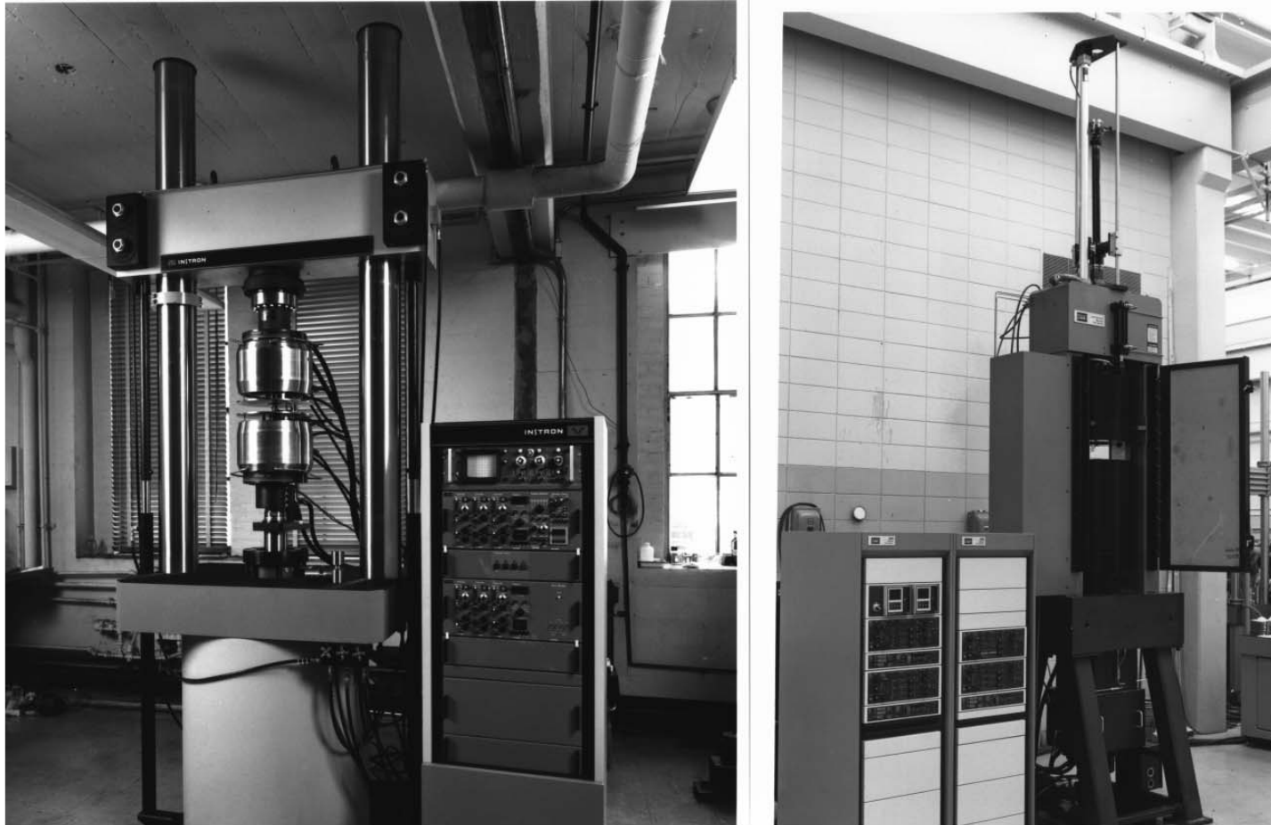
FIGURE 10.2.3.2(c) Three-dimensional axial/torsion pressure testing systems.
